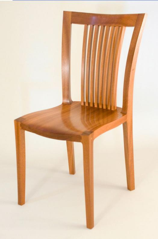
This project was an exercise in using compound curves to produce a chair with a pleasing, comfortable shape. The construction is a mix of template routed legs, back slats, and the seat blank's side profile. The seat blanks were tapered and glued with a stepped offset between each one to produce the side-to-side curvature. The seat was then hand faired smooth to produce the compound curves in the seat. The finish is a wipe-on varnish and oil mix.
